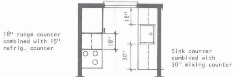
Fig. 14 Kitchens for 1-bedroom living units (with minimum storage, counter area, fixtures). For kitchens for 0-bedroom living units, see pp. 27-28.
